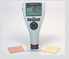
SIDSP® eddy current sensors are applicable to a wide range of non-ferrous substrate materials with various conductivities such as copper, titanium, etc. without the need of recalibrating the gauge to the particular substrate.
